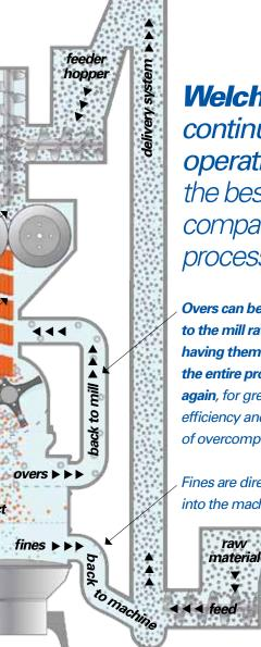
WelchDry's continuous operation is the best roller compaction process
